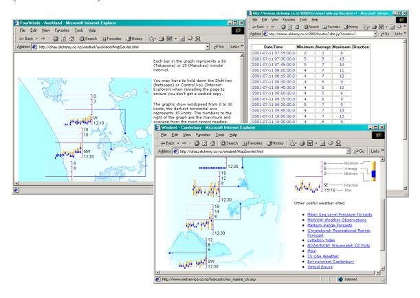
The system was based on Java 2 technologies and was heavily distributed. Radio modems at locations around the coast sent packets to a relay station which then forwarded them to a base station. The base station then used Java Messaging Service and Comm APIs to communicate data to the Windnet server. The server can receive data from multiple base stations via JMS messages.
