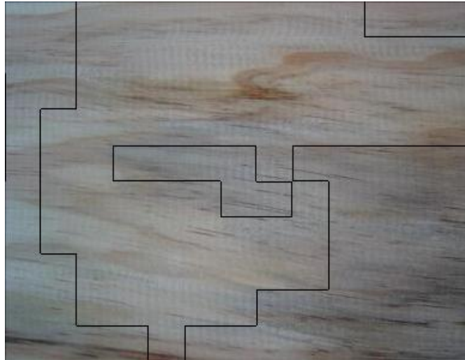
Fig. 5. An board cutting example based on sapstain classification.
