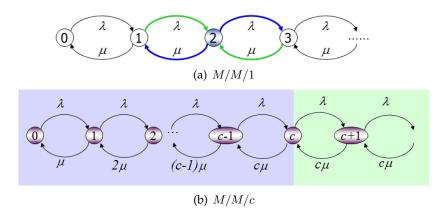
Fig. 3. Markov chain diagrams used to explain the queueing models of (a) M/M/1, and (b) M/M/c.
