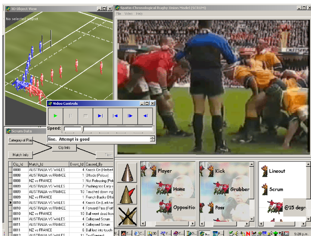
Figure 9: A screen shot from SCRUM, with the pseudo-3D spatial representation (with superimposed scrum and player objects) on the top left; video clip database is bottom left; video is top-right; object hierarchy is bottom-right.
