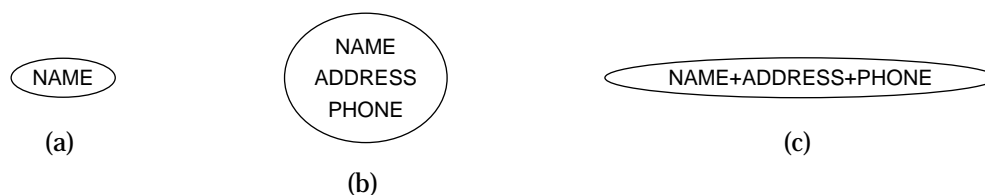
Figure 2: (a) A bubble that contains a single attribute; (b), (c) bubbles that contain multiple attributes
