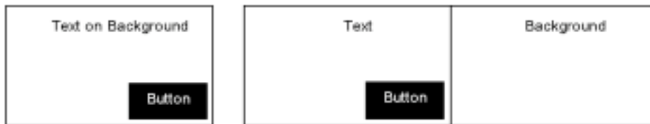
Fig. 1. System design for the standard single layered display (left) and the MLD TM (right)
