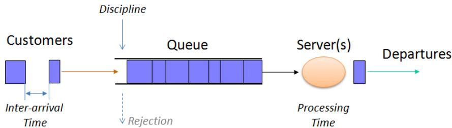
Fig. 1. Diagram of a simple queueing system.
